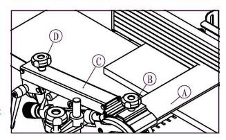
The height of the knife shaft cover (A) is carried out through the star screw (D).
