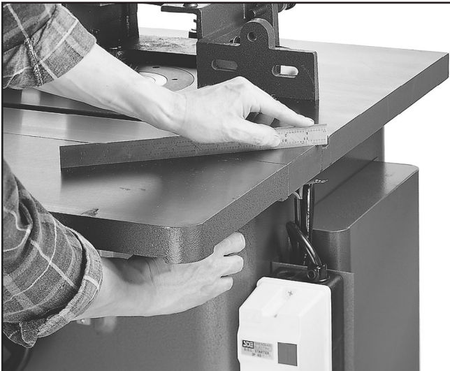
Figure 9. Adjusting to ensure flatness.
