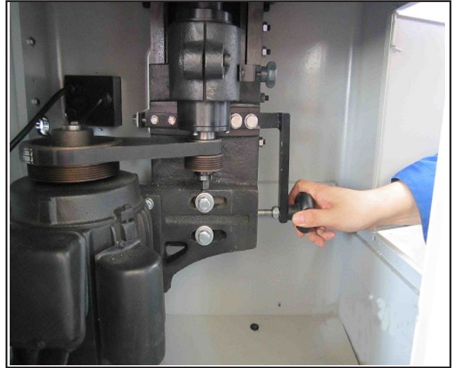
Figure 13. Adjusting the V-belt tension
