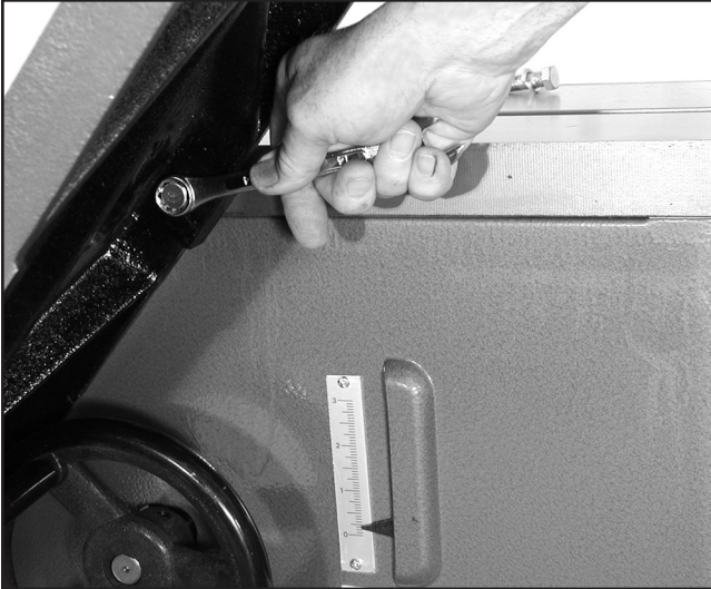
Figure 8. Installing extension wing.
